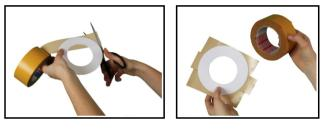
Turn around the cardboard ring with the film covered side facing upward and lay it back onto the Kleenex. Stick the second cardboard ring against it. Now you have created a round film-holder with AstroSolar Film cleanly and securely fastened without cheases and ripples – but most of all: without stressing the film!
