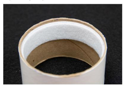
In order to start making a solar filter for your telescope, camera lens, or binoculars, we need to make a cylinder that will fit around the dew shield or lens hood. This cylinder will hold the solar film in place and fit snugly around your optics.
